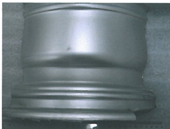
1#-3 Specimen before test
