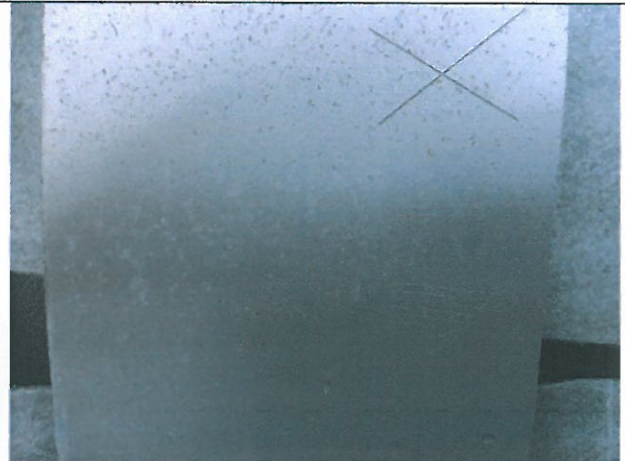
1#-1 Specimen after test(384h)
